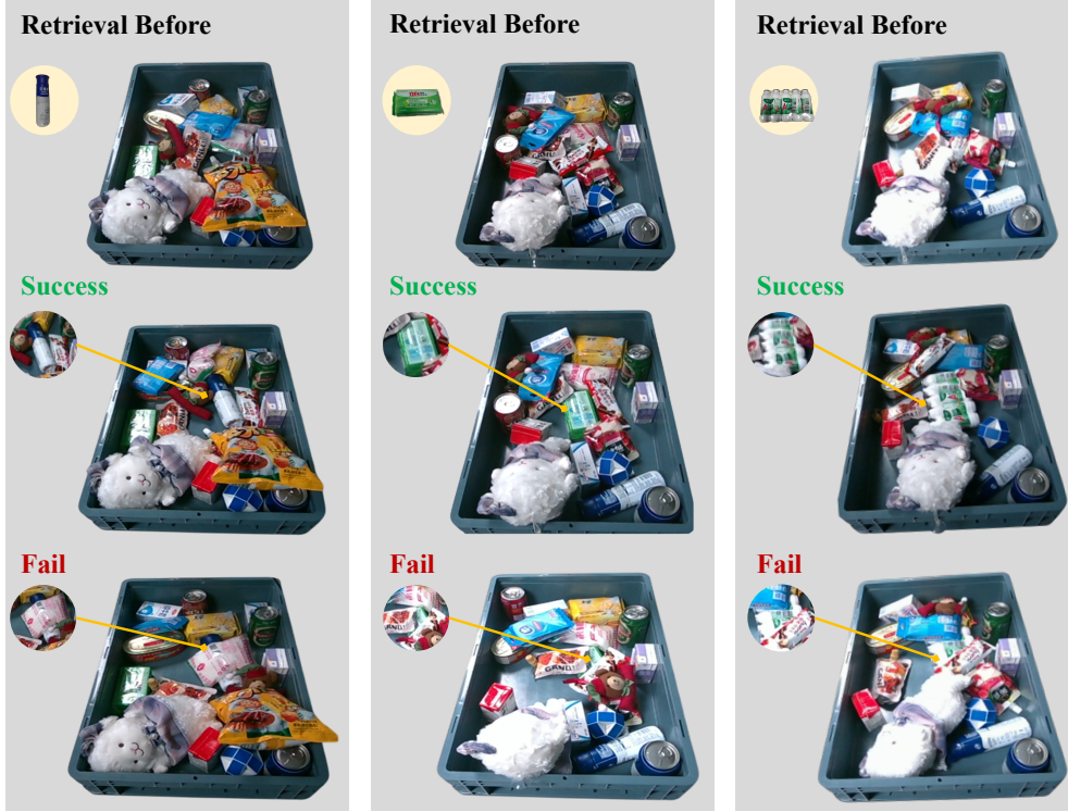
Figure 6: Examples of successful and failed object retrievals on the real robot.
